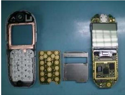
Photo 2.10 Keypad PCB and Shield removing
