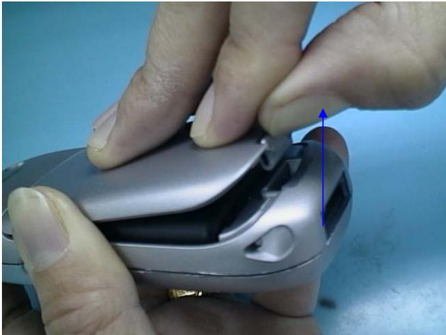
Photo 2.3 Battery cover removing
