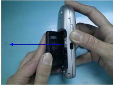
Photo 2.5 Battery Removing
