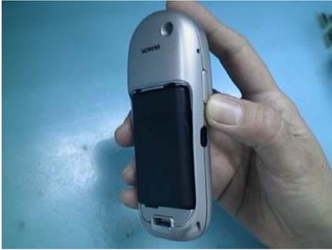
Photo 2.4. Battery compartment
