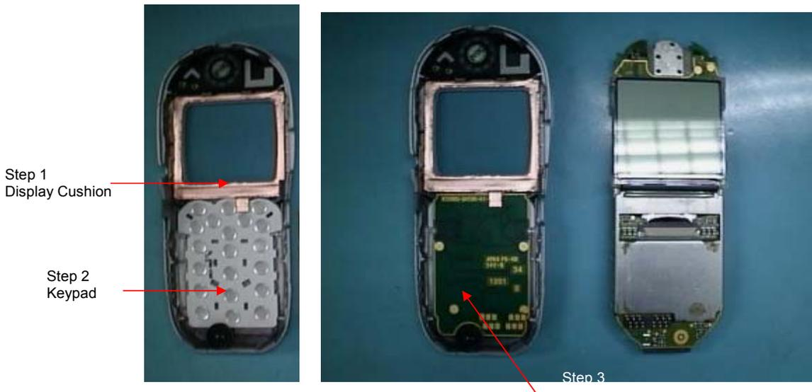
Photo 2.20 Keypad and Display cushion assembly
